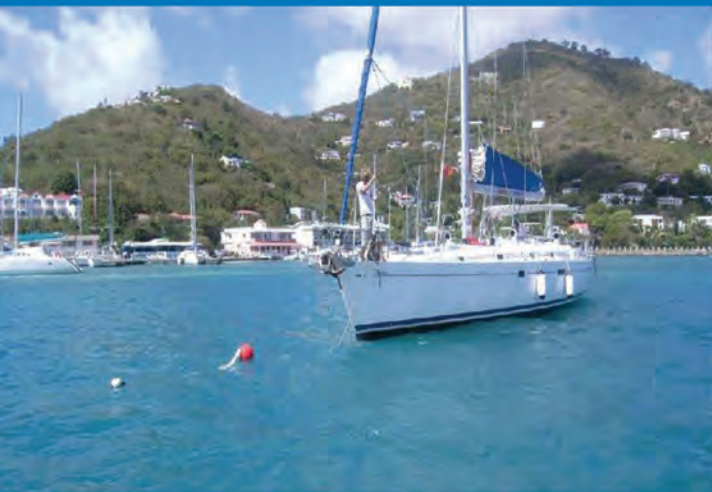
1. Approach red mooring buoy with pick up line and float
